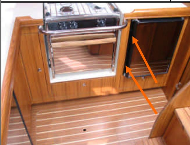
Fig.8 secure the ring mounting holes to freezer wood face trim. using 4 pieces #10 x 3/4" long Oval head self tapping screws.
