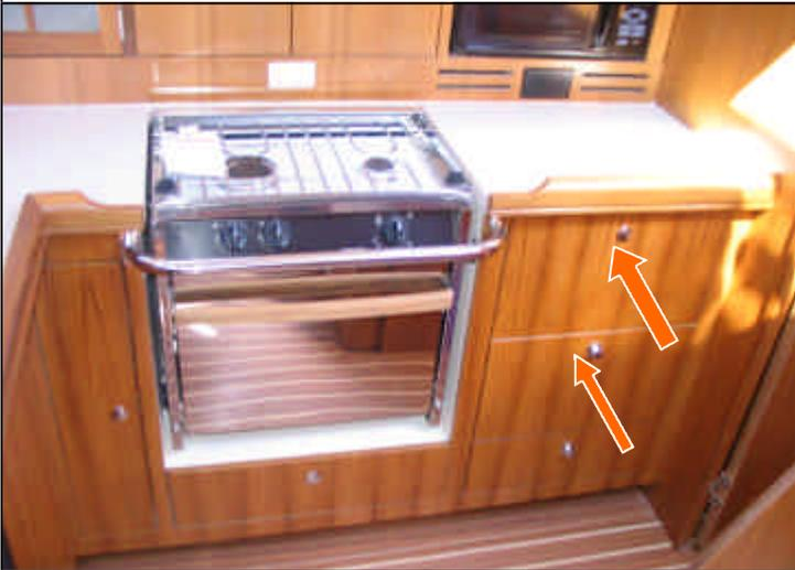
Fig.1 Remove middle & upper drawer from galley
