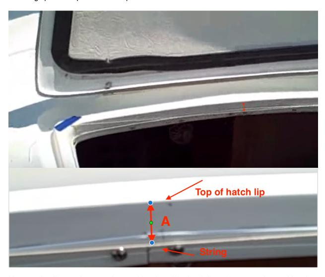
Measure the distance between the out side edge of the hatch lip on the port to the outside edge on the starboard. See B below.
